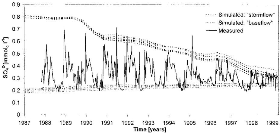
**Fig. 3** Measured sulphate concentration in the catchment runoff (biweekly intervals), and simulated sulphate concentration in groundwater for flowpath lengths  $\leq 150$  m ("stormflow") and  $>150$  m ("baseflow"), respectively, (annual mean values; 10 replicates each to account for spatial heterogeneity of sorption isotherms).
