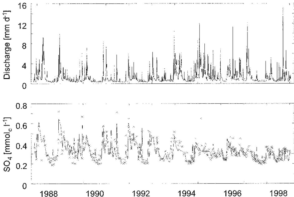
**Fig. 2** Time series of discharge (upper panel), observed (x) and simulated (black line) sulphate concentration in the Lehstenbach catchment runoff.
