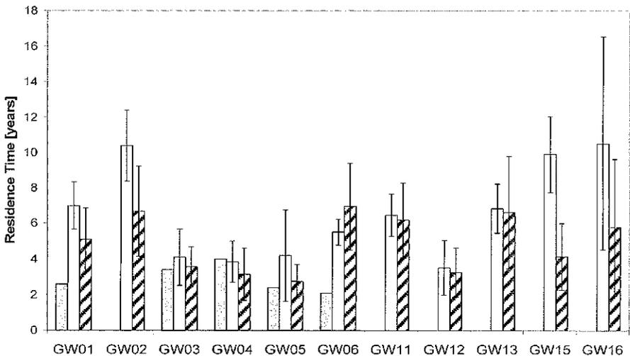
**Fig. 1** Mean groundwater age measured by  $^{18}\text{O}$  (Zahn, 1995) (solid grey column) and simulated for varying hydraulic conductivity (white column) and varying thickness of the aquifer (hatched column). For simulated data, mean values and standard deviations (10 model realizations each) are given.
