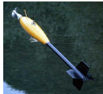
12 cm diameter rotor mounted on the sinker (55 kg)
