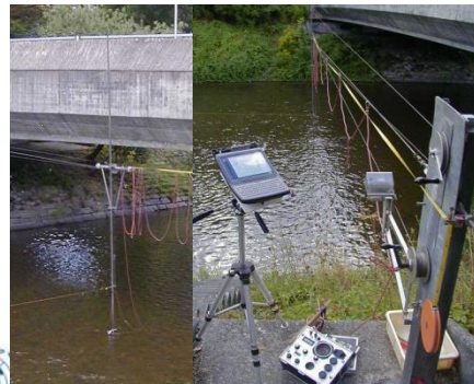
Current meter 8 cm diameter mounted on a bar transported by a cable way.
