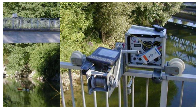
Current meter 12 cm diameter mounted on a sinker from a bridge.
